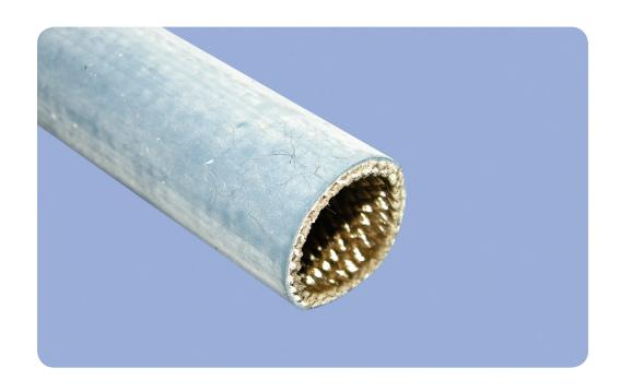
**Ben-Har**<sup>™</sup> **1151-FRB Grade A** is a rugged, flame-retardant, silicone rubber coated sleeving that provides excellent cut-through and abrasion protection for wiring systems in applications with temperatures ranging from -70°C to +200°C. Because the specially formulated silicone rubber is extrusion coated over the non-combustible fiberglass braid, it results in a reinforced sleeving that is superior to ordinary dip-coated sleeving and unreinforced rubber or plastic tubing.
