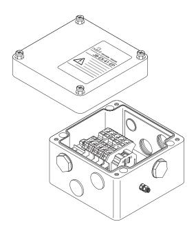
Industrial polyester junction box with earth plate for use in hazardous areas. This box can be used to make connections between power cables, heating cables and cold lead cables using M25 metallic connection kits or glands. Earthing of the connections is realized via the earth plate
