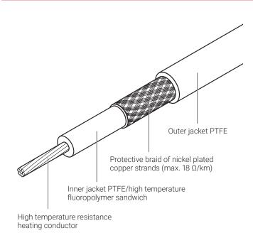
nVent RAYCHEM XPI is a polymer insulated (PI) series heating cable, suitable for use in hazardous areas. It has been designed for use in freeze protection and temperature maintenance applications of pipes, tanks and other equipment. XPI offers an economical solution for a wide variety of heat-tracing applications, in particular for pipe lengths beyond the maximum circuit lengths of parallel heating cables.
