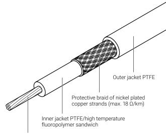
High temperature resistance heating conductor
