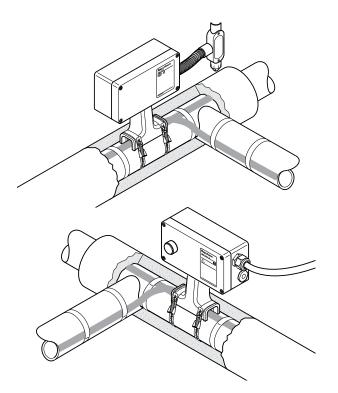
The nVent RAYCHEM JBM-100 kit is designed to connect power to up to three nVent RAYCHEM BTV, QTVR, XTV, KTV, or VPL industrial parallel heating cables and is approved by FM, CSA, and PTB for use in hazardous locations.
