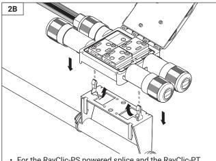
For the RayClic-PS powered splice and the RayClic-PT powered tee, fold up two center snaps, then position the connector over the snaps and press down.
