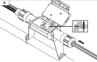
• Insert prepared heating cable end into connector. Push until heating cable is fully inserted and end is visible through opening in connection cover plate.
