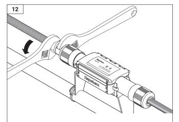
· Using two wrenches, attach user-supplied 1/2-inch conduit. To avoid breaking housing, do not exceed 15 ft-lbs of torque. Broken connectors must be replaced.
