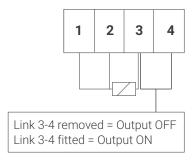
Terminals 1 to 3 allow for the connection of a three wire PT100 sensor.
