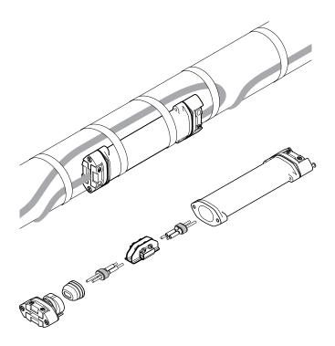
The nVent RAYCHEM S-150 is a cold applied low profile splice for in-line connection. This universal kit fits with all nVent RAYCHEM industrial heating cables, BTV, QTVR, XTV and KTV, meaning simplified product selection and reduced inventory to stock. It can be used in applications with temperatures ranging from  $-50^{\circ}$ C to  $215^{\circ}$ C. It is approved for use in hazardous areas.
