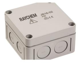
nVent RAYCHEM JB16-02 and JB-82 temperature-resistant polycarbonate junction boxes for non-hazardous areas. For use with nVent RAYCHEM self-regulating heating cables, to make a power connection, tee, splice, powered splice/tee. Up to four heating cables, or three heating cables and the appropriate size power cable can be connected through the four entries and connected to the rail mounted terminals.
