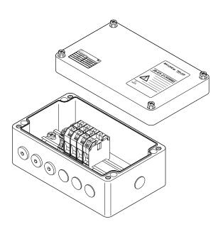
Industrial junction box for use in hazardous areas with PI and MI heating cables when large terminal sizes are required. This box can be used to make connections between power cables, heating cables and cold lead cables. Depending on the configuration of the system, the box can accommodate multiple heating cables/cold leads and a power cable.
